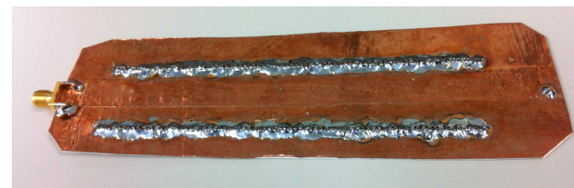
SLOTTED WAVEGUIDE ANTENNA
